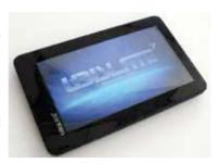
Aakash is a 7-inch touch screen with ARM 11 processor and 256MB RAM, running Android 2.2 OS. Aakash 1 was developed with an aim to reach 25,000 colleges and 400 universities across India and provide all students at least one computing device, as part of the "One Laptop per Child (OLPC)" scheme.
