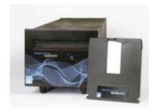
The first working prototype of a holographic storage system is called Tapestry. However, the technology is yet to become a reality since InPhase Technologies, the company working on Holographic Storage filed for bankruptcy in 2011 and can't make it ready for mass market due to technological constraints and hence is open only for organisational usage.
